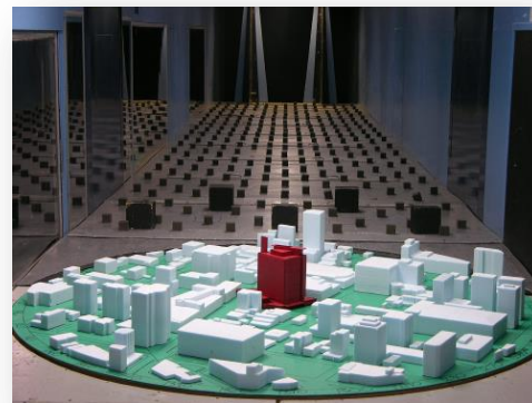
Example of scale models in one of RWDI's boundary layer wind tunnels.
